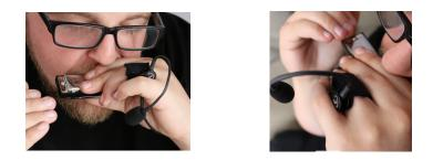
The "Feather" is mounted by using the patented "Saddle-Clip" (provided). One side of the Saddle-Clip is used to hold Saddle-Clip to the finger wrap and the other side of it is to saddle/hold the "Feather" securely in place. Adjust the Flexible Micro-Gooseneck to your desired position and you are ready to plug in. Experiment with different locations for the sound you desire. Most people prefer to have the pickup element about 2 to 3 inches from where the sound is produced.
